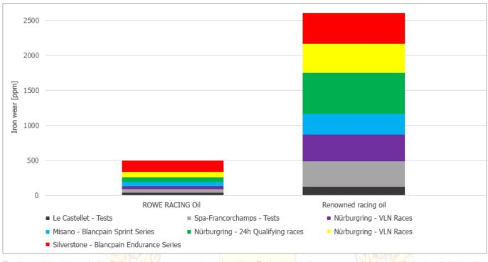
The diagram (above) shows the iron wear accumulated over several races/test drives. The iron already shows more wear with the renowned racing oil after the third run (right) than it does with the ROWE RACING oil (left) after all 7 races / test drives together.
